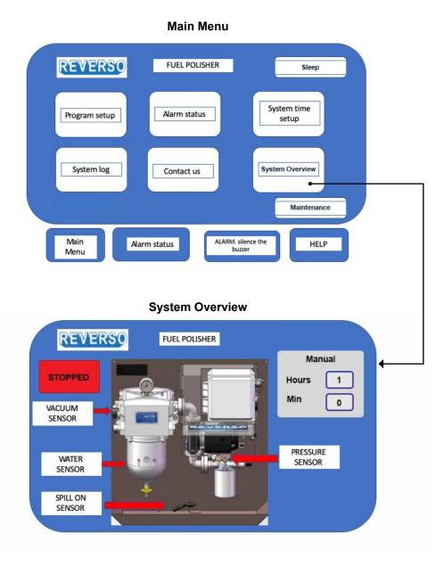
Note: Marine Fuel Polishing Systems (FPS models), do not include pressure sensor and spill sensor.
