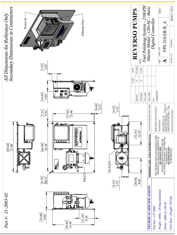
Dimensions are the same for 220V AC, and versions with touchscreen or mechanical control panels.
