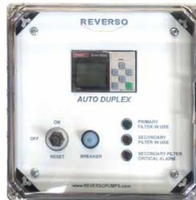
Status lights indicate which filter is in use and when the backup filter is in need of maintenance. The NEMA DC controller manages the switch-over. Should there be a loss of power, the user can manually turn the red handle atop the unit to conduct the switch to the secondary filter.
